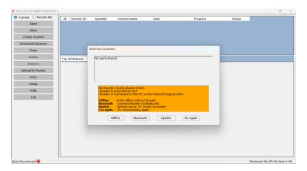
Check the port and physical connections between the reader, cable and PC.
